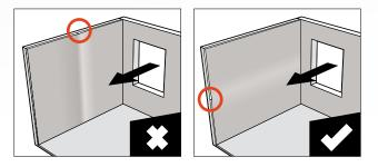
With horizontal fixing, there is only one joint which is below eye level.
